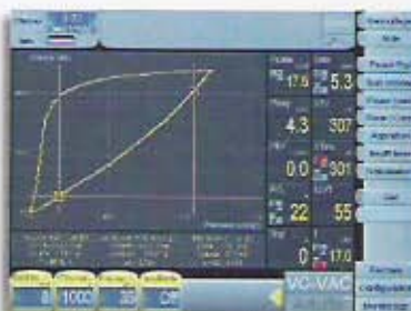
Pressure/volume curve with low inflation flow method
