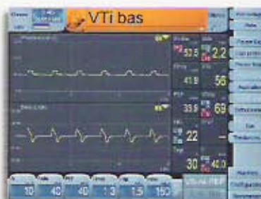
Possibility of adjusting PEEP up to 40 cm H 2 O
